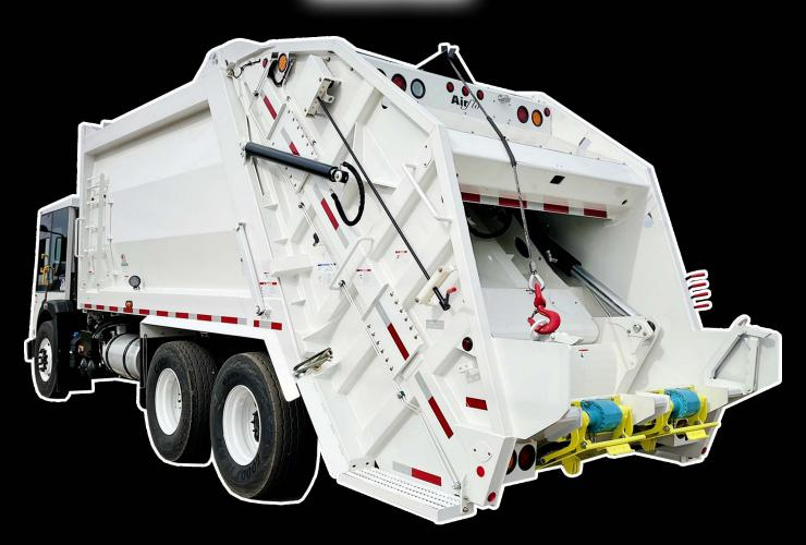
DESIGNED WITH ONE-PIECE BODY SIDE CONSTRUCTION FOR SUPERIOR STRENGTH AND STREAMLINED APPEARANCE, THE UNI-MAX® IS CONSTRUCTED WITH ABRASION RESISTANT HARDOX® WEAR PLATE, MAKING IT THE STRONGEST STEEL SPEC IN THE INDUSTRY
